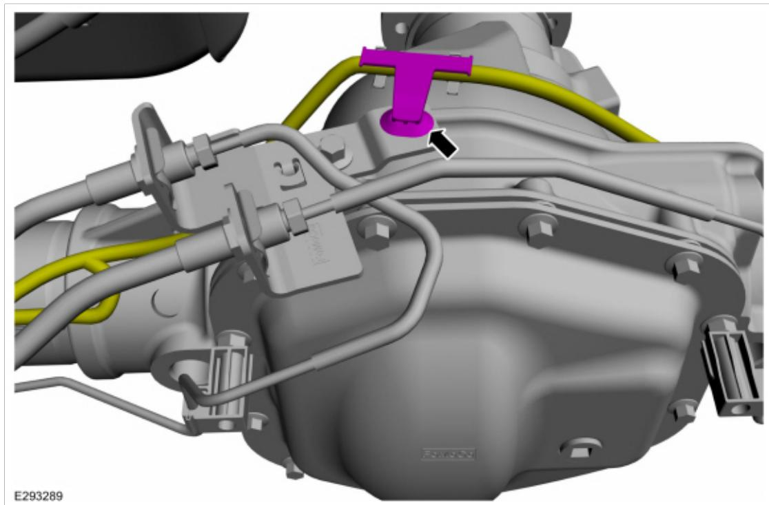
2. Disconnect the 2 brake tube fittings.
