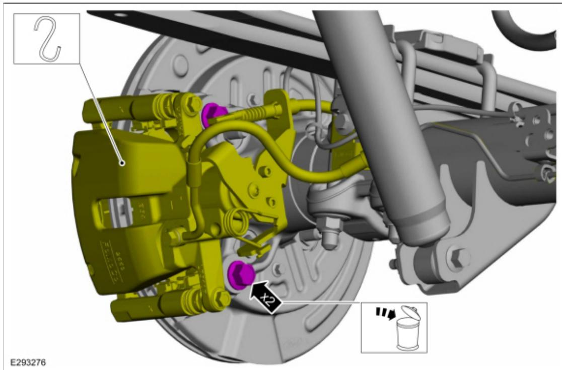
3. Remove the brake disc.
