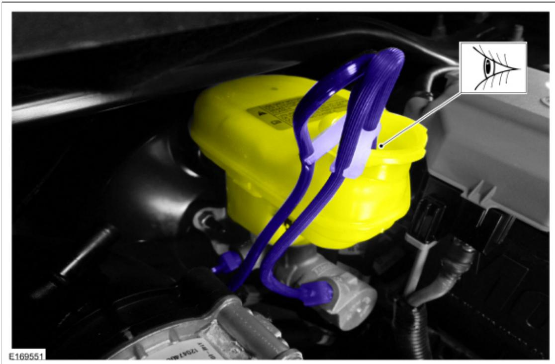
5. Have an assistant pump the brake pedal slowly until clear bubble free fluid flows from the brake tubes.
