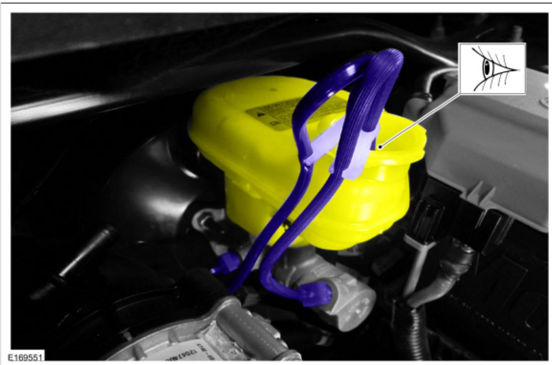
7. Tighten the brake tube fittings.
