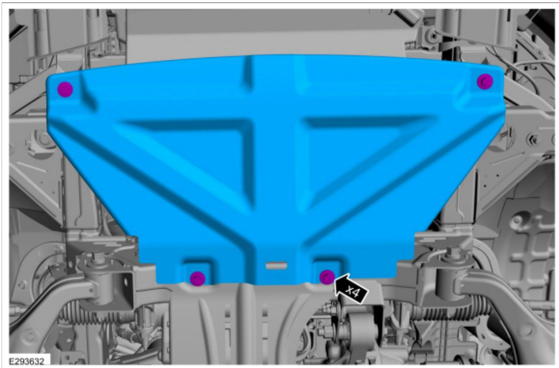
3. Remove the bolts and the front axle skid plate.
