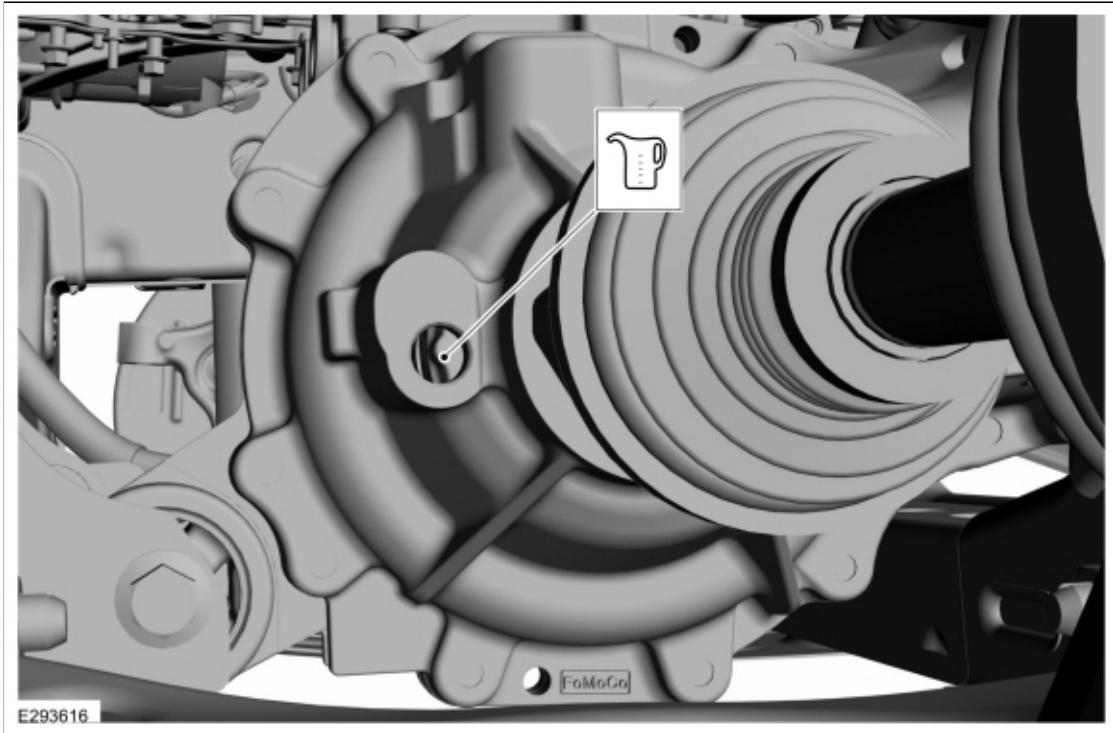
4. Install the front differential fill plug.
