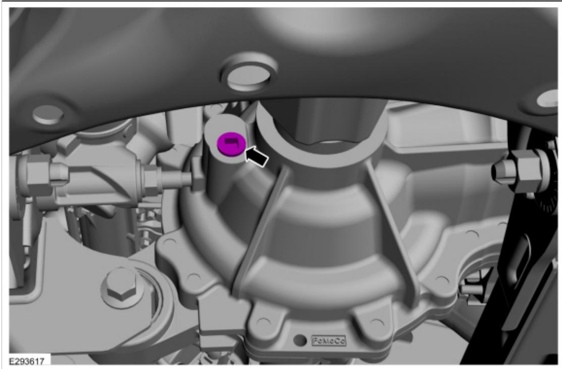
3. Check and top off the differential with clean differential gear lubricant. The differential gear lubricant level should be to the bottom of fluid fill plug opening.
