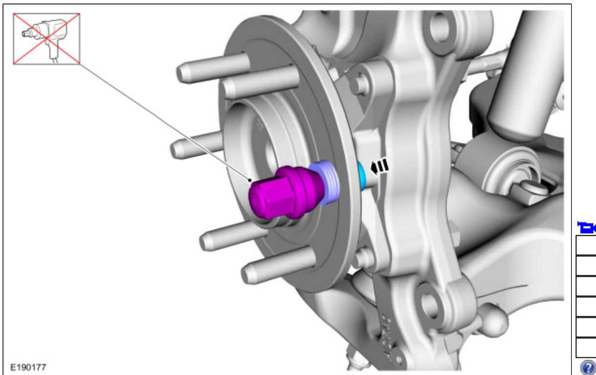
2. Install the brake disc shield.
