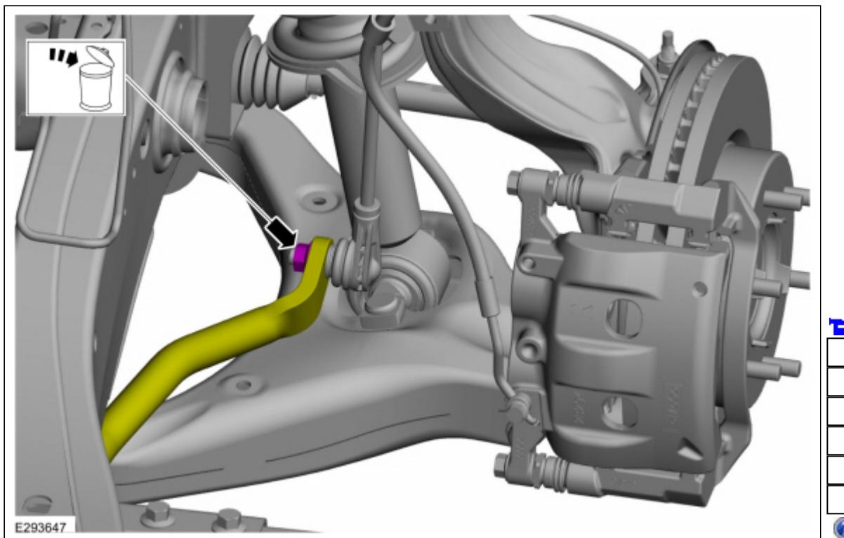
3. **NOTICE:** To prevent the stabilizer bar from moving freely in the suspension system, increasing the possibility of contacting or damaging surrounding components such as the tires or front driveshaft; the raised ring on the stabilizer bar must be secured in the inner groove of the stabilizer bar bushing on the driver's side of the vehicle.
