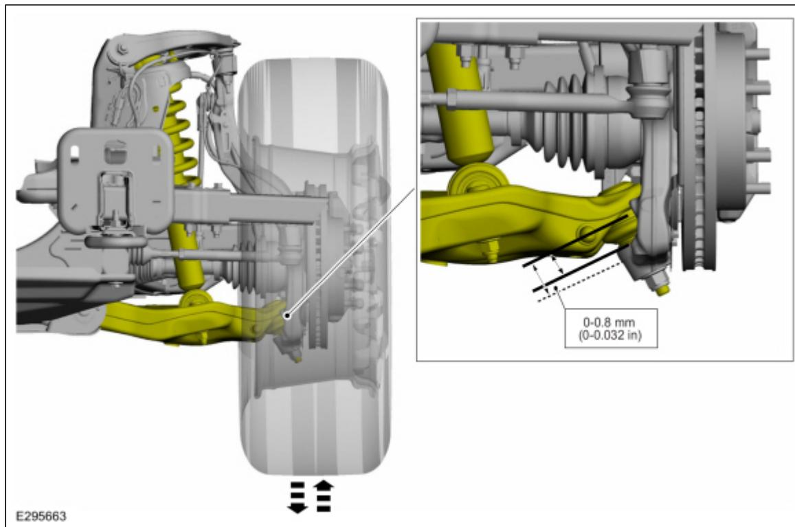
6. Measure the ball joint deflection while an assistant pushes up and pulls down on the lower control arm, by hand.
