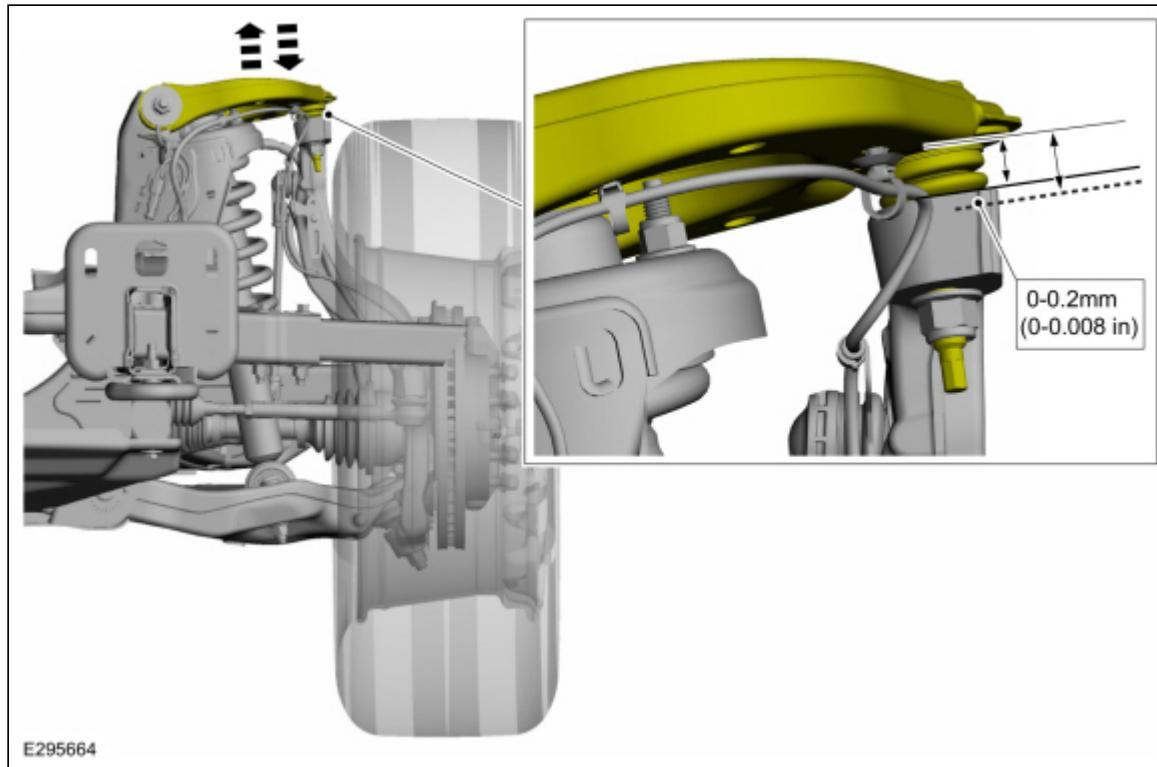
9. Measure the ball joint deflection while an assistant pushes up and then pulls down on the upper control arm, by hand.
