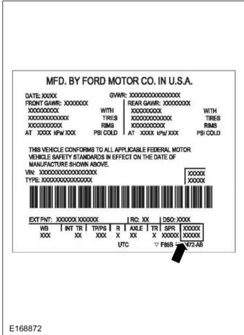
**NOTE:** Powertrain calibration information is limited to a maximum of 5 characters per line on the VC label. Because of this, calibration identification consisting of more than 5 characters will wrap to the second line on the VC label.
