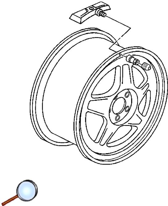
**Note:** If any tire sealant is noted upon tire dismounting, replace the sensor. Refer to [Tire Pressure Indicator Sensor Replacement](#). Also remove all residual liquid sealant from the inside of the tire and wheel surfaces.
